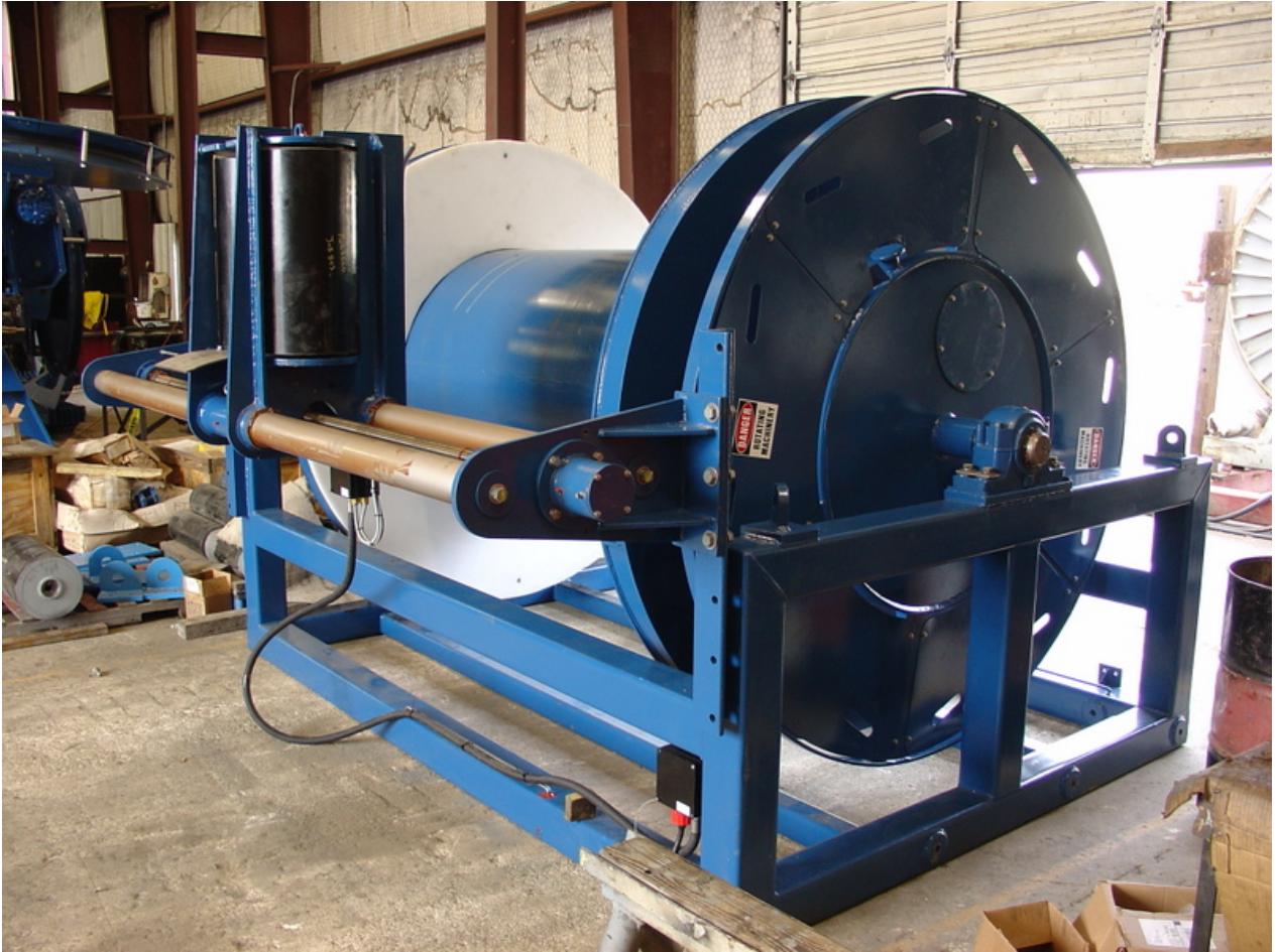
MOOS Winch with level wind attached. Note lifting eyes at corners of winch stand.
