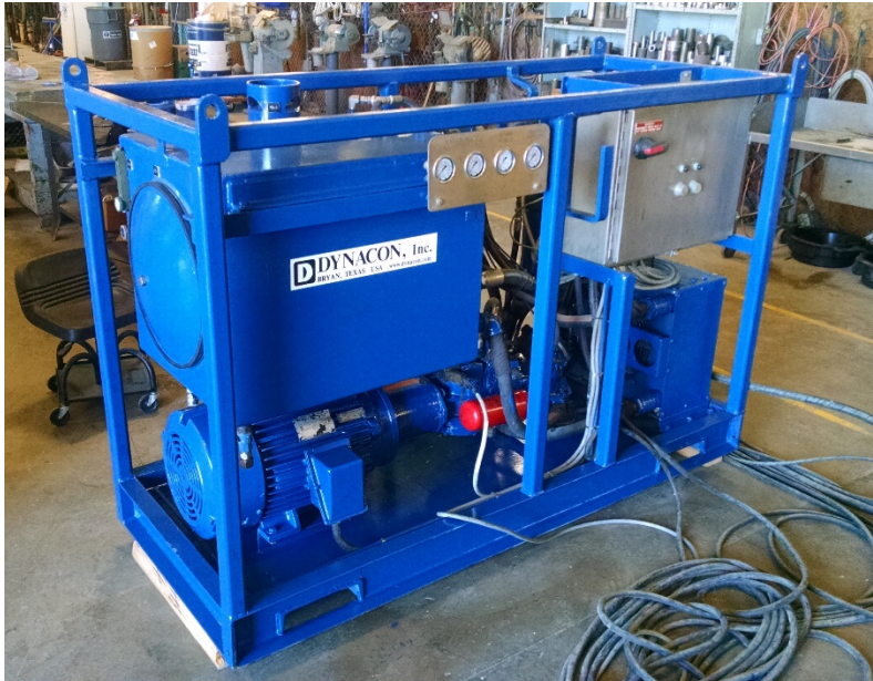
Hydraulic power unit (HPU).
